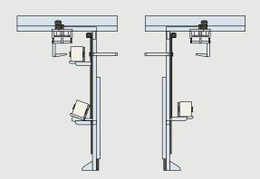
The lifting device picks up the twisted packages from the output conveyor belt of the cabling machine. It delivers the packages to the transport system and transports them to the next location for subsequent processing.
