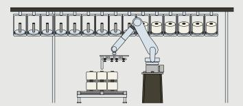
The depalletiser takes up the supply packages in order to load them onto the transport system fully automatically. The empty tubes are removed at the same time.
