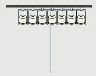
The supply package transport system replaces the conventional high/low creel. It precisely delivers the packages for a complete machine side.
