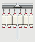
The roving bobbin transport system delivers the bobbins from the roving frame to the spinning machine. Semi-automatic or fully automatic systems are available.
