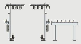
The lifting device takes up the cones from the conveyor belt of either the winding machine, the rotor-spinning machine or the air-spinning machine, and delivers them to the next process step.
