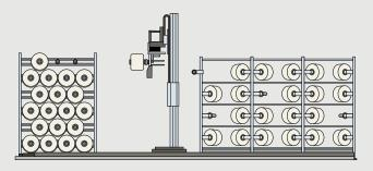
A linear 3-axis robot picks up the packages from the rack and transfers them precisely to their positions at the heatset creel.
