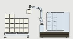
The robot AGV picks up the packages from a pallet or from the conveyor belt of the machine and stores them in its internal buffer system. Then it transports the packages and loads the subsequent machine.
