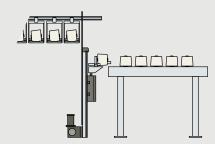
Complete twist packages are removed from the twisting machine via a rail system for further downstream processing.
